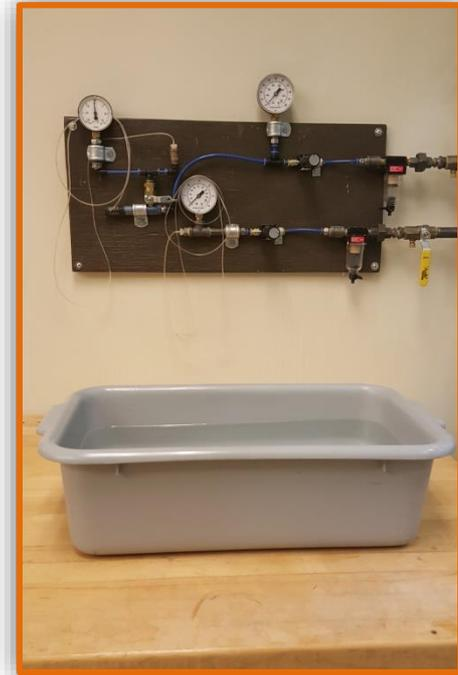
Pressure/Vacuum leak station
