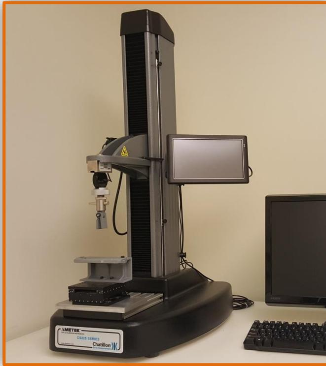
Mechanical force gage and test stand
